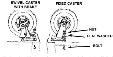
Turn your equipment table upside down. Install the 2 swivel casters on the end of the table with the handle using 8 bolts, flat washers and nuts.
