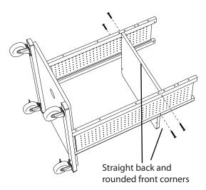
Step 2: Using the small Allen wrench(O), install the middle shelf(F) with 4 - M6x35 Allen screws(G).
