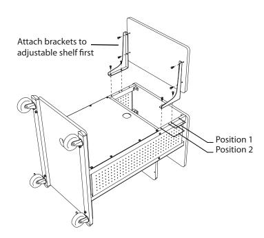
Step 5: Using the small Allen wrench, install the adjustable shelf(C) to the brackets(D) and legs with 8 - M6x10 Allen screws(J). **Tighten all screws down.**
