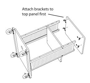
Step 3: Using the small Allen wrench, install the top(A) to the legs with 4 - small L brackets(B) and 8 - M6x10 Allen screws(J).
