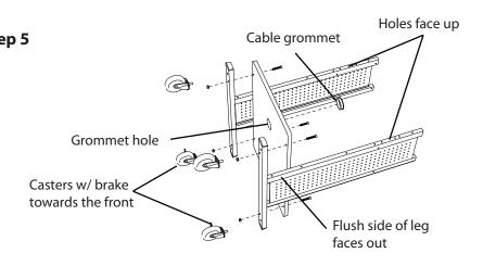
Step 1: Using the large Allen wrench(P), install the base panel(M.) to the legs(H) with 4 - M10x35 Allen screws(K) and nuts(L). Install the Casters(N) and tighten with the caster wrench. Install the cable grommet(I), and cover remaining holes with the small grommets(Q) and sticker(R).
