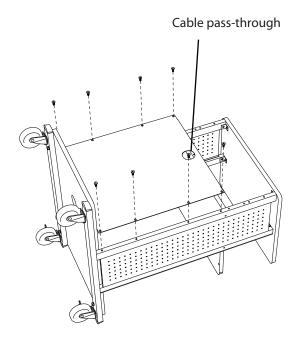
Step 4: Using the small Allen wrench, install the back panel(E) to the legs with 8 - M6x10 Allen screws(J).
