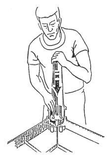
1. Place the table top upsidedown on a raised surface for convenient assembly. Slide each table leg into it's proper groove by applying gentle downward force. (LEFT)
