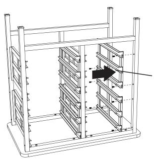
Step 2: Screw Certwood rails to the legs with M6 x 10 Flat Phillips screws.
