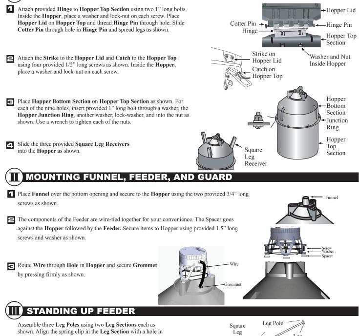
shown. Align the spring clip in the **Leg Section** with a hole in the other **Leg Section**. Attach provided **Feeder Feet** to bottom of **Leg Poles** as shown. Lay Hopper on side. Install a **Leg Pole** on the inside of each of the **Square Leg Receivers**. With two **Leg Poles** against the ground as shown, carefully stand up the **Feeder** assembly.
