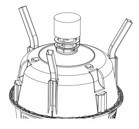
Slide the three provided Square Leg Receivers into the Hopper as shown.
