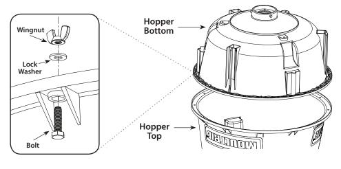
Connect Quick Lock Feeder Kit to assembled Hopper as shown.
