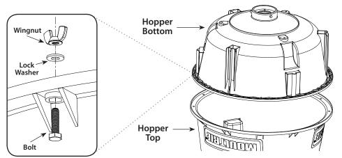
Connect Quick Lock Feeder Kit to assembled Hopper as shown.
