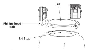
Install **Lid** by aligning handles with notches in **Hopper Top**. Twist until Lid rests flush against Lid Stop.
