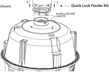
Slide the three provided **Square Leg Receivers** into the **Hopper** as shown.
