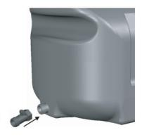
Shut-Off Valve shown in closed position
