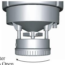
**Rotate Counter** Clockwise to Open
