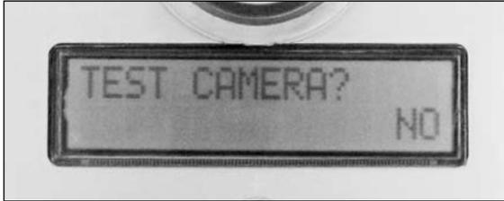
This option allows you to run a diagnostic test on the BirdCam. It is used to check the BirdCam's functionality and verify that it is working properly. During this test, important subsystems are tested. This setting has two options:
