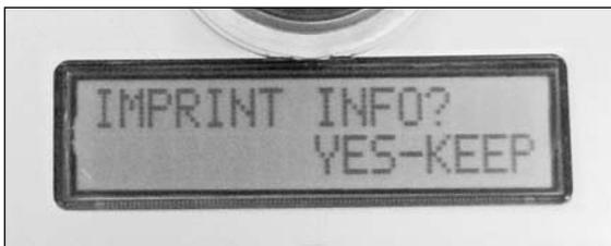
**YES-KEEP** – This option is the default factory value and simplifies the SETUP menu. The imprint information that is currently programmed into the BirdCam will appear in a databar at the bottom of your photos. This selection allows you to bypass the time, date, and BirdCam name programming screens.
